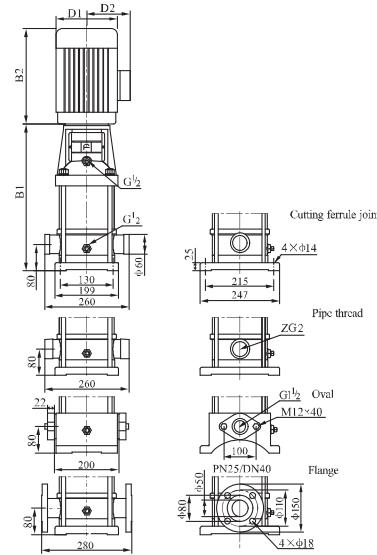
CDL10-16~10-22 sub-connection of pipeline has no oval flange connection.
