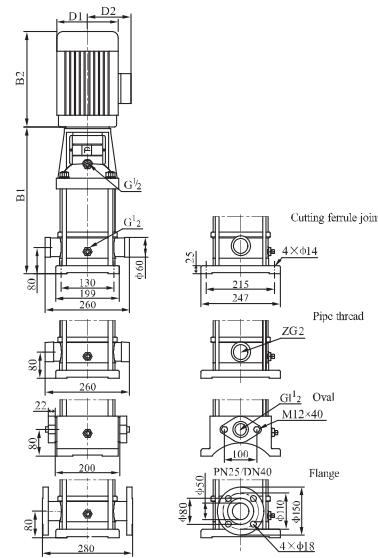
CDL8-14 ~ 20 sub-connection of pipeline has no oval flange connection.
