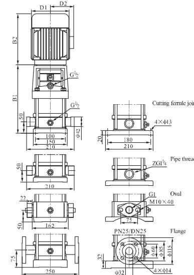
CDL3-25 ~ 3-36 sub-connection of pipeline has no oval flange connection.
