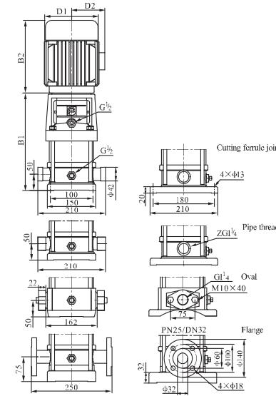
CDL5-26~5-36 sub-connection of pipeline has no oval flange connection.
