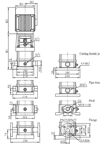
CDL2-18 ~ 26 sub-connection of pipeline has no oval flange connection.
