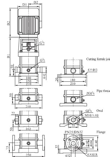
CDL4-19 ~ 4-22 sub-connection of pipeline has no oval flange connection.
